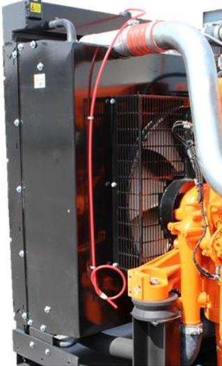
The radiator is mounted on the base frame to avoid vibrations coming from the engine.
